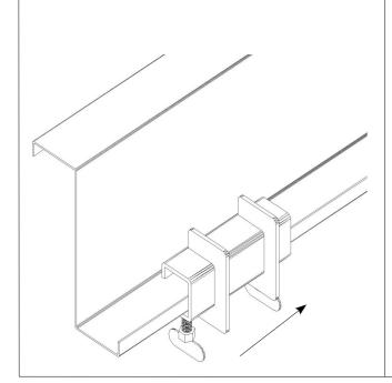
**Step – 2**Slide Support bar into the End Clamp and tighten both wing bolts.
