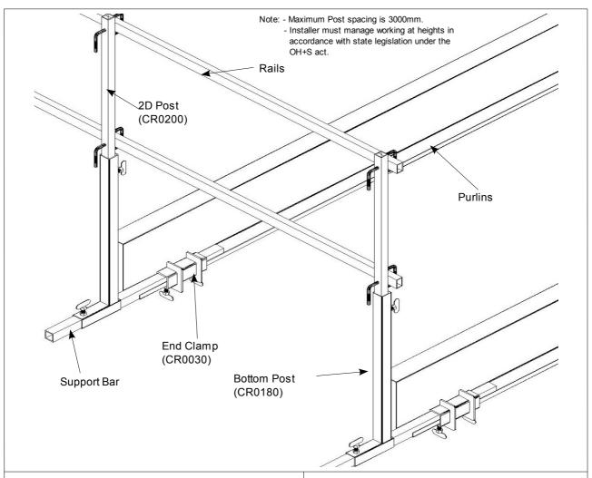
**Step – 1**Position the End Clamp on the purlin.
