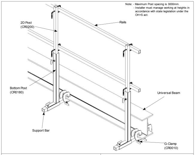
**Step – 1**Position the G-Clamps onto each side of Universal Beam.
